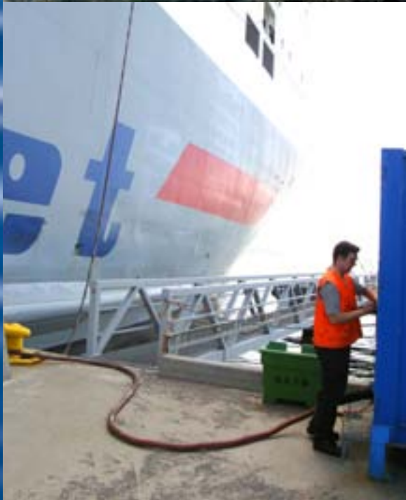
Connecting a Ro/ro-vessel in Port of Göteborg
